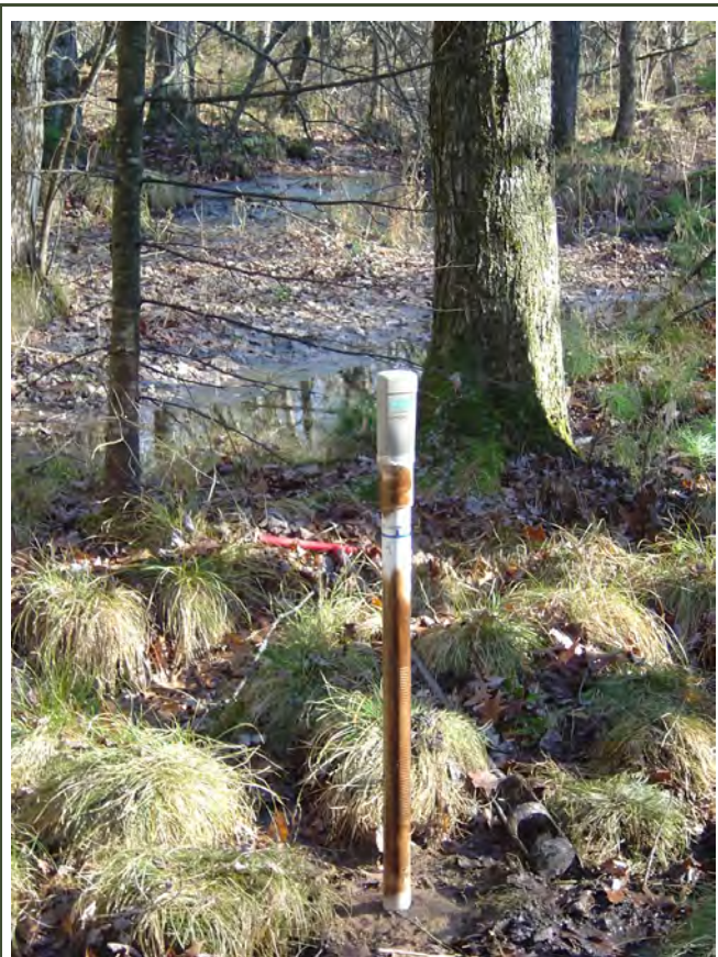
Figure 2.16 Automated monitoring well installed near the inflow of a lotic headwater red maple swamp along an unnamed tributary to Ashokan Reservoir.
