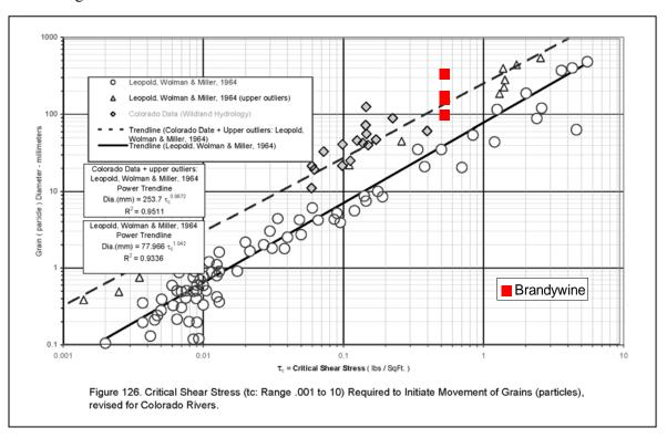
Figure 8. Shields Curve Diagram showing Brandywine critical shear stress calculations for each monitoring year.
