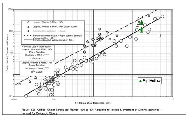
Figure 10. Shields Curve Diagram showing Big Hollow critical shear stress calculations for each monitoring year.
