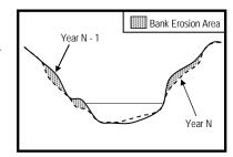
Figure 3. Determining bank erosion area for Year N.
