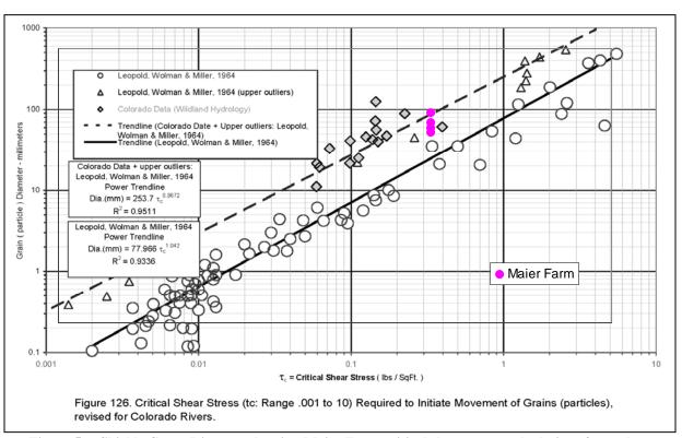
Figure 5. Shields Curve Diagram showing Maier Farm critical shear stress calculations for each monitoring year.
