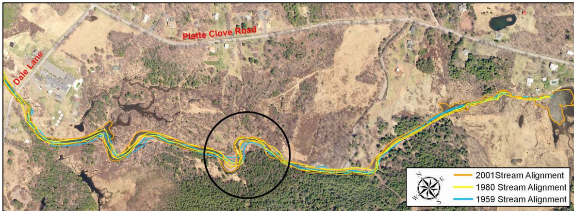
Historic stream channel alignments beginning at Station 157400 overlaid with 2006 aerial photograph
