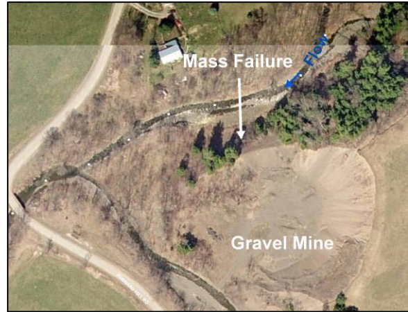
Mass Failure at Stations 39532 - 39316
