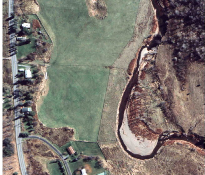
Figure IV-33: In this field in Ashland behind Carrington Road, note the absence of riparian vegetation along the fields. The GCSWCD has measured migrations of this meander bend of over 40 feet in a single storm event.
