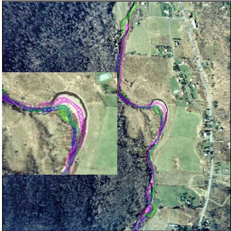
Figure III-13: Lateral migration of meander bend in Ashland as shown in 1959 (blue), 1995 (purple) and 2000 (photo).
