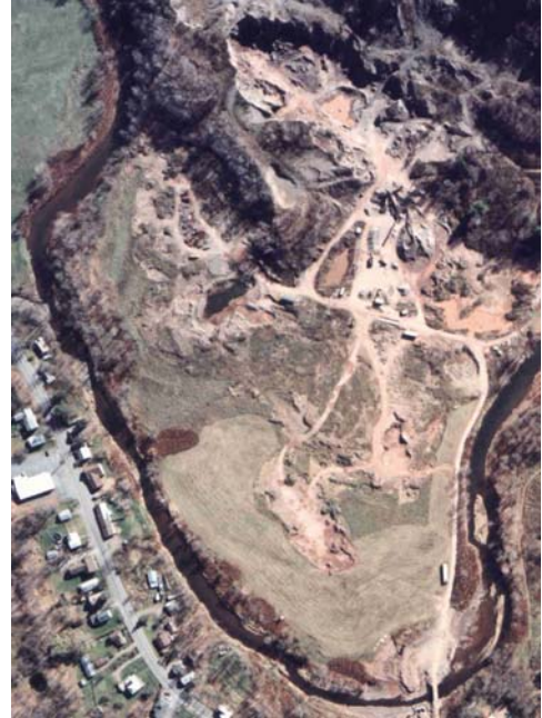
Figure IV-13: Glacial deposits of gravelly loam are desirable for fill as seen in this view of Tompkin's Quarry.
