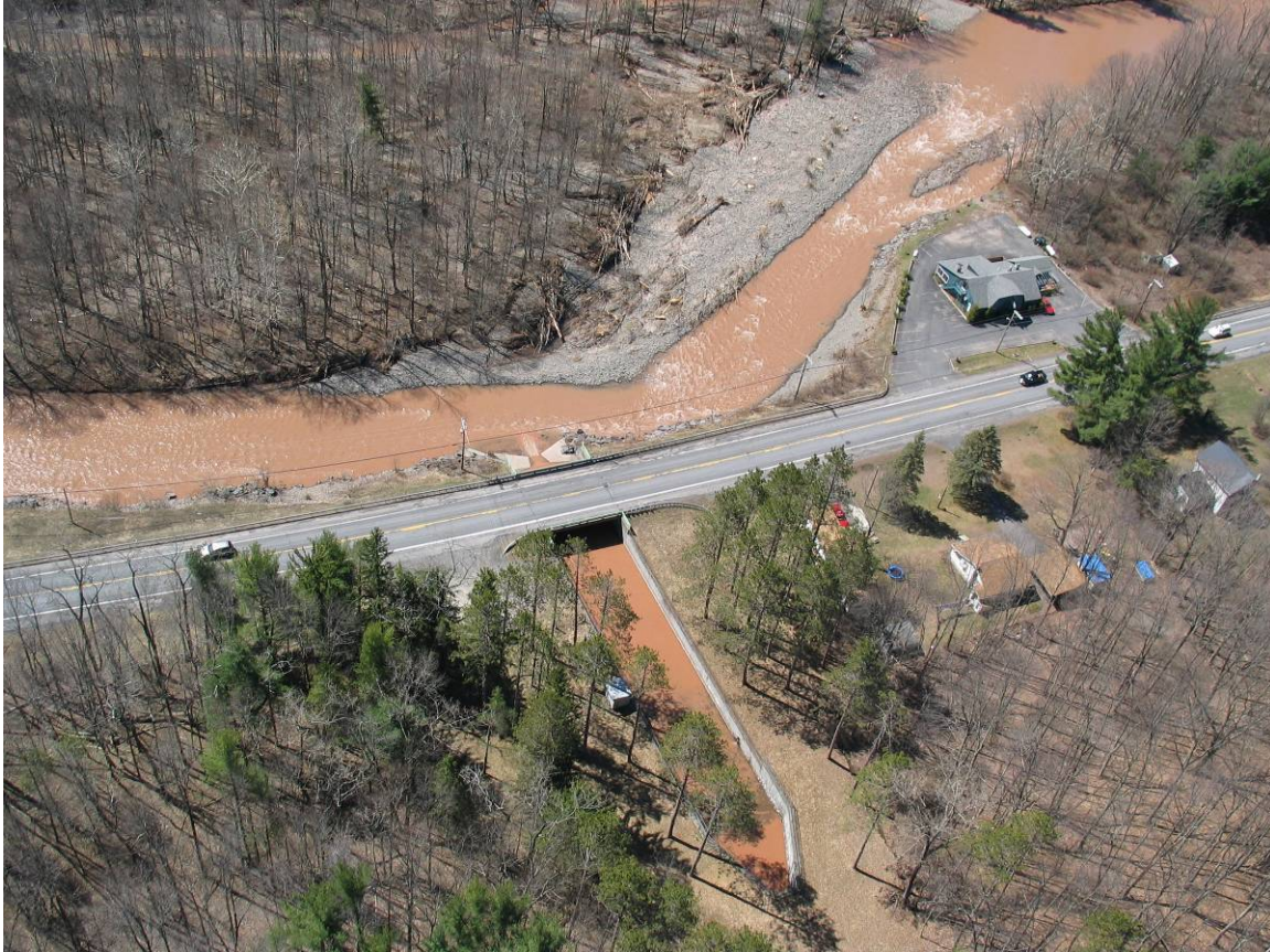
Figure 1.3. Shandaken Tunnel Outlet (Portal) discharging turbid water to a turbid Esopus Creek following the April 2-3, 2005 flooding.
